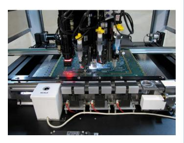
Proprietary FLOware® software controls all aspects of system operation and even handles the control of Pickand-Place tools for special applications. All systems are configured with ease-of-operation in mind using auto vision, auto XYZ nozzle calibration, a nozzle cleaner, and tool-less Taper-Lock™ mounting hardware. These features ensure a consistent set up and process with minimal operator intervention.
