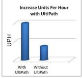
After the first dispense pass, UltiPath monitors its internal timers and determines which component is ready for its next operation. By selecting the next dispense operation based on a constantly monitored time sequence, UltiPath maximizes gantry effectiveness.
