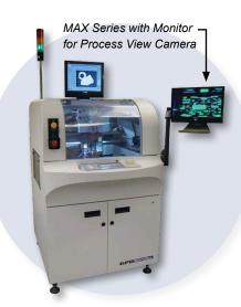
Process View Camera is compatible will all needle dispense processes. It may be retrofitted to existing installed systems. Also, for machines configured with Process View, video capture may also be added separately. Couple this inspection method with our gantry mapping process - Contour Mapping™which is performed on all GPD Global® dispensers, and our high-resolution, encoded drive motors, and it is easy to see why GPD Global® is a leader in high precision, high accuracy dispensing systems.
